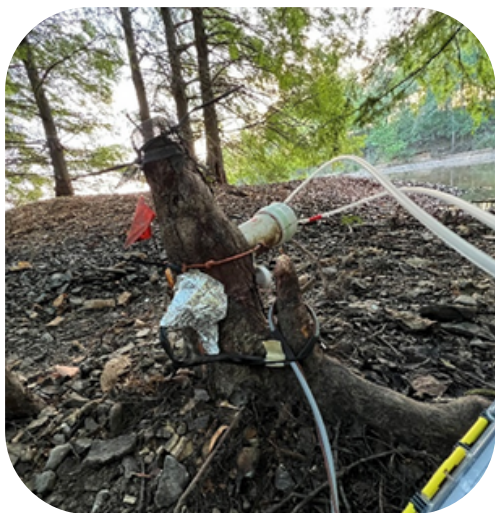
Methane emissions and sap flux being measured from a knee at HBS (photo by Dr. J.B. Moon).
