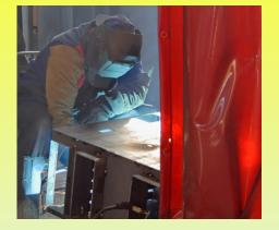
A welding curtain shields employees from the direct rays of arc welding and cutting operations.
