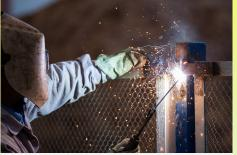
Arc welding and cutting uses an electric arc between a metal electrode and a base material to join or cut metal.
