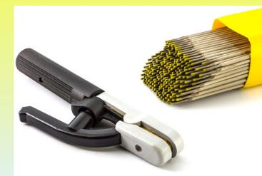
The welder inserts one of these electrodes (right) into the electrode holder (left).
