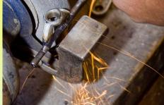
**Grinding** uses a grinding wheel that rotates at high speed to cut metal.
