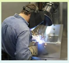
A welder uses a local exhaust duct to quickly remove toxic fumes and gases.
